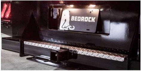
Integrated 2" receiver hitch rated at 18,000 lbs.
