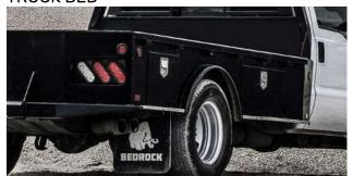
Full steel frame with 4" & 3" structural C-channel construction & 1/8" steel diamond plate deck
