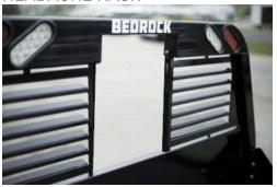
Patented adjustable headache rack provides the perfect fit for your truck
